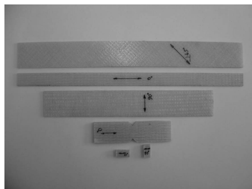
Fig. 2. Specimens for mechanical properties of the glass fiber-epoxy composite material.
