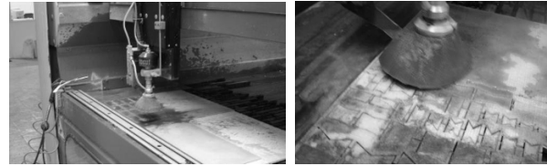
Fig. 5. Cutting specimens using water jet.
